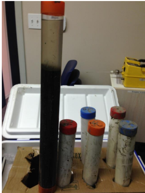
Photo 8: Sediment core samples in capped tubes ready for extruding and sampling
