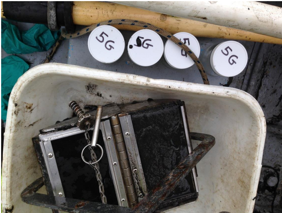
Photo 7: Petite Ponar (top) sampler used for surface sediment grab sampling
